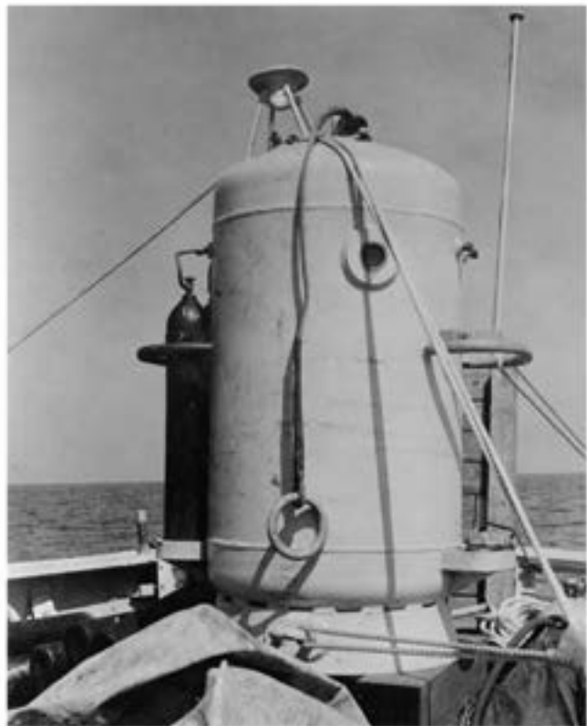
U.S. Navy Historical Center images show a 1939 McCann rescue chamber similar to the one used in the U.S.S. Squalus rescue, and a cutaway illustration of the space inside.
